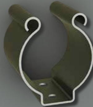
CAD-design for reproduction of grenade holders in turret basket
