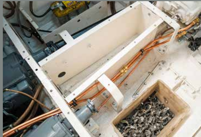
CAD-design rear storage box
